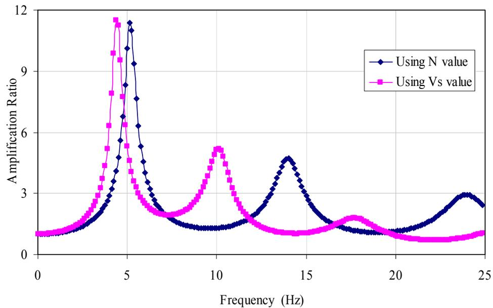
**Figure 20:** Typical amplification ratio using MASW and SPT
