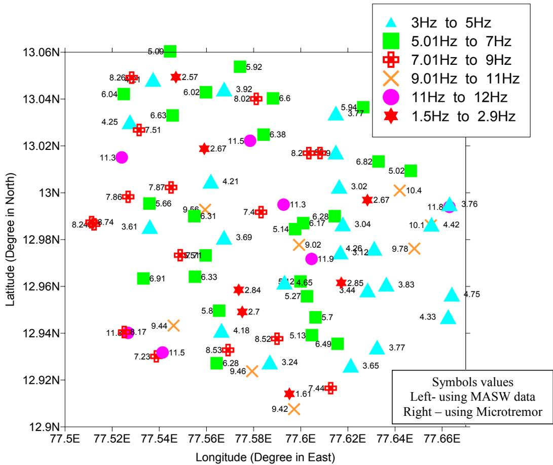
**Figure 23:** Predominant frequency from microtremor and site response using shear wave velocity
