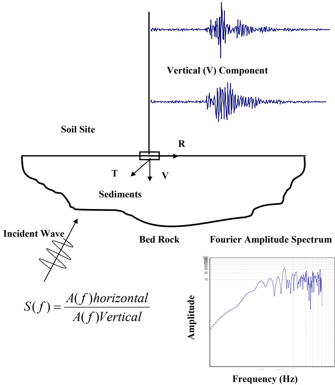
Figure 21: Horizontal to vertical spectral ratio technique – Layout
