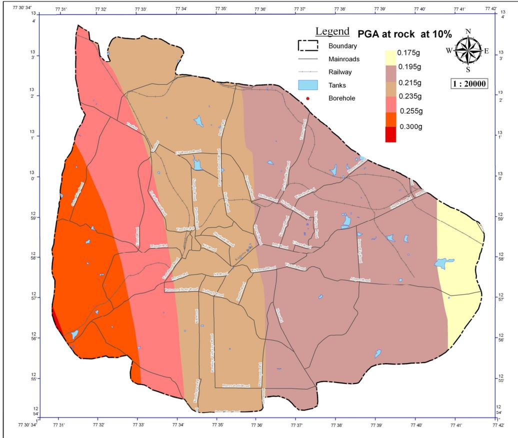
**Figure 13:** Peak ground acceleration contours at rock level with 10% probability of exceedance in 50 years.
