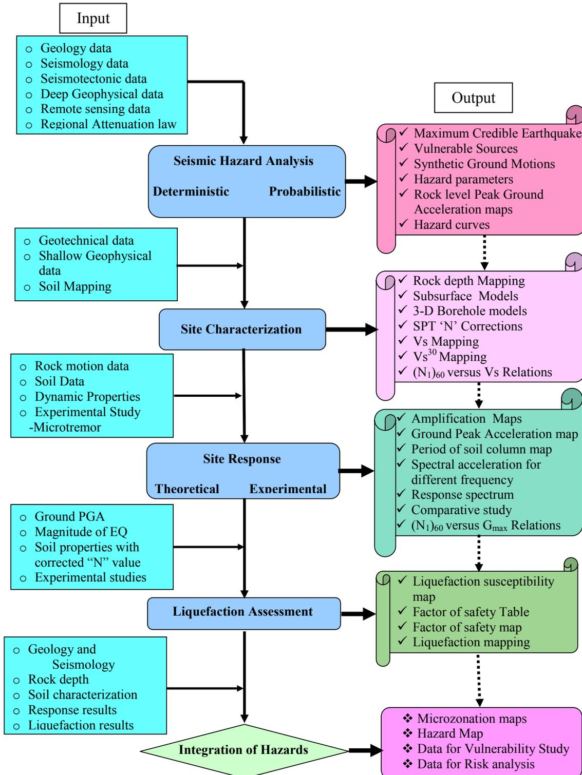
Figure 7: Flow chart for seismic microzonation
