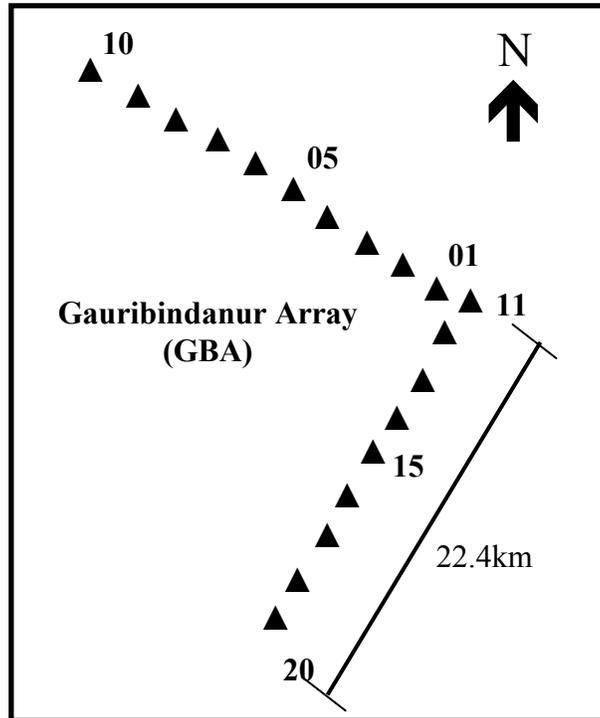
**Figure 8:** Pattern of the location of receivers in Gauribindanur Array.
