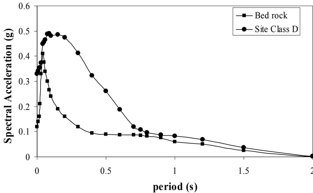
**Figure 25:** Uniform hazard response spectrum for bed rock and site class D with 10% probability of exceedance in 50 years (5% damping) for Bangalore.
