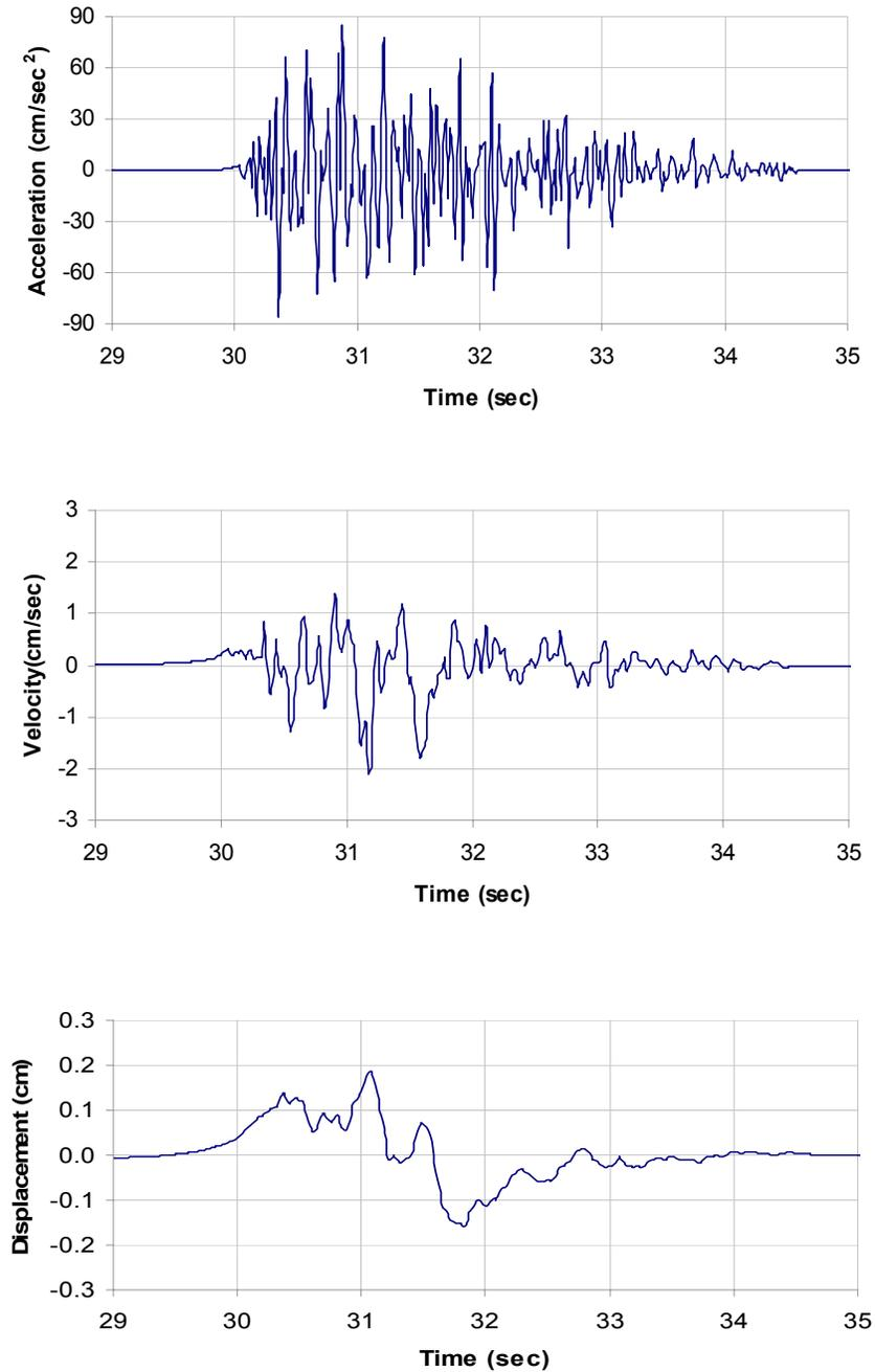
**Figure 16:** Typical Input Ground Motion used for analysis
