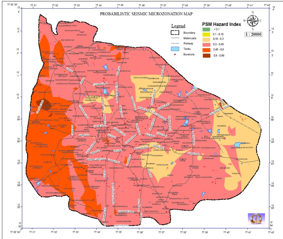
Figure 34: Probabilistic seismic microzonation map
