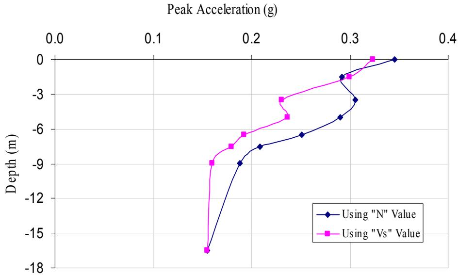
**Figure 19:** Typical peak ground acceleration with soil column thickness
