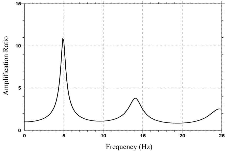
**Figure 17 (c):** Amplification Spectrum between the bedrock and ground surface
