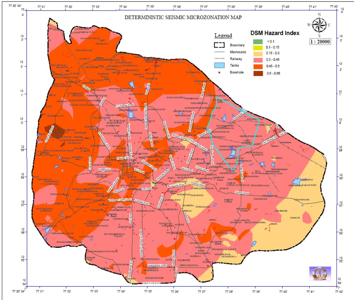
Figure 33: Deterministic seismic microzonation map
