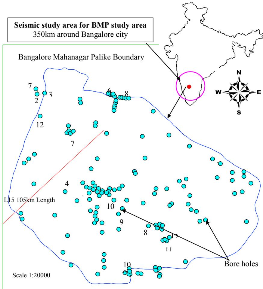
**Figure 6:** Study with borehole locations used for site response study
