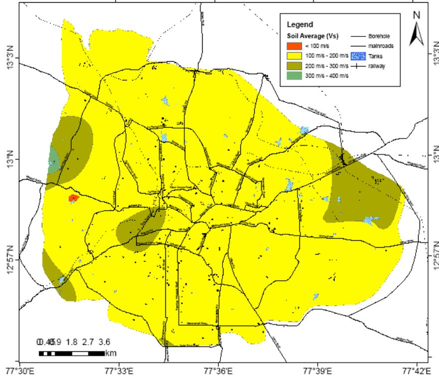
**Figure 16:** Equivalent shear wave velocity for soil
