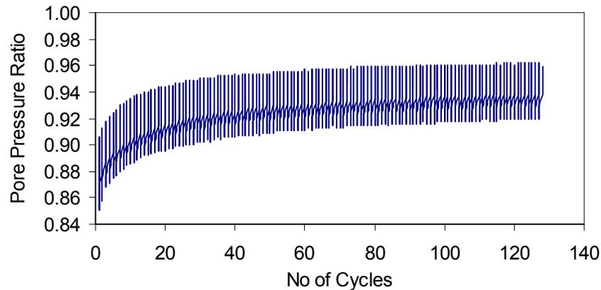
**Figure 29:** Typical pore pressure ratio plots with no of cycles
