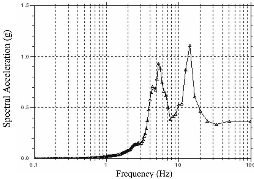
**Figure 17(b):** Response Spectrum for 5% damping at Ground surface
