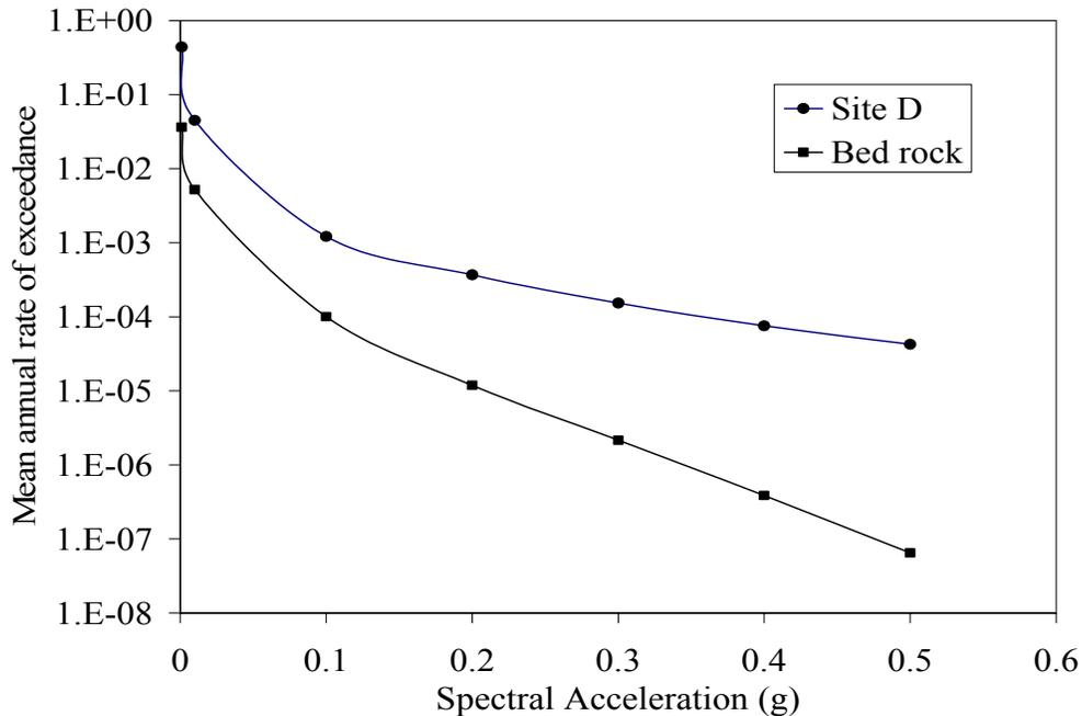
**Figure 24:** Spectral acceleration at bed rock and site D corresponding to period of 1s and 5% damping for Bangalore.
