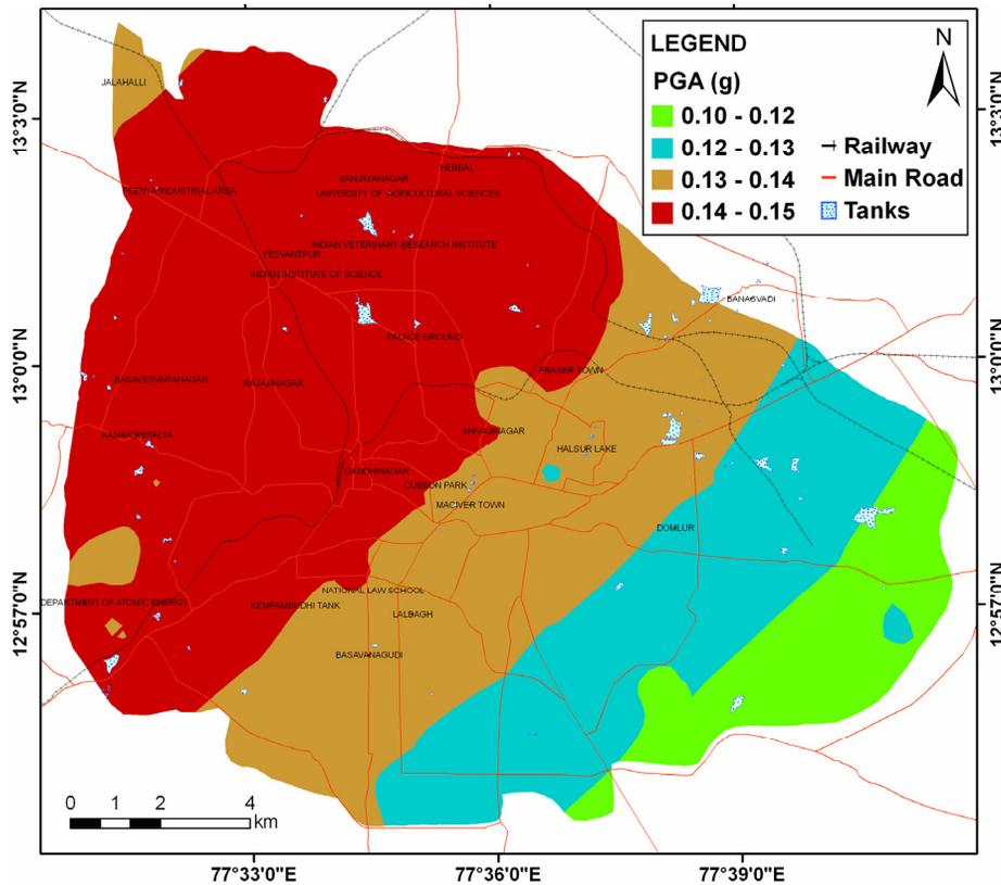
**Figure 10: Peak ground acceleration map using DSHA**
